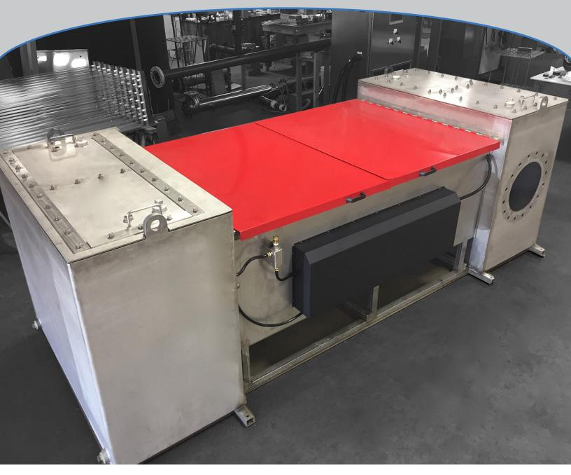
**NONCON-5000-6-8 x 30** Installation. 2.5 MGD wastewater disinfection plant with 100% redundancy. The reactor is designed as a "U" allowing for a smaller footprint. Remote Ballast Control Center with PLC and touch screen operator user interface.
