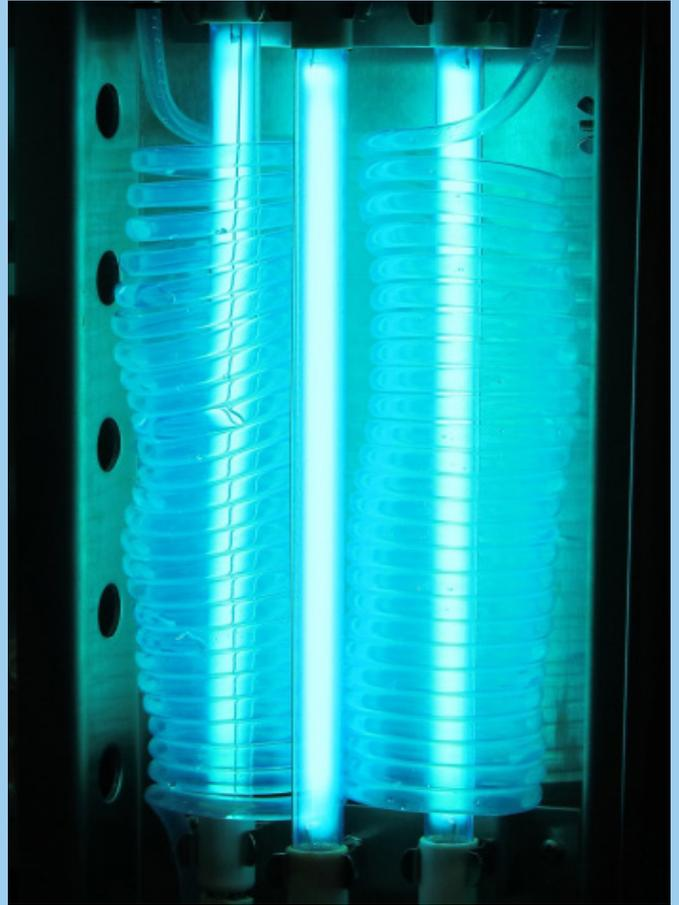
Once in the enclosure, the system is fan cooled to ensure optimum UV lamp performance.
