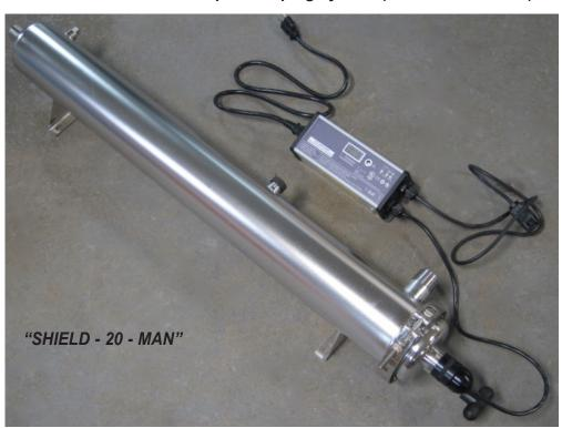
The GUV SHIELD MAN system comes with an integral manual quartz sleeve wiping system. A manual wiping system helps remove build up on the protective quartz sleeve. Fouling occurs when the water has impurities like minerals. High iron and hard water can coat the quartz sleeve and interfere with the proper transmission of UV light.
